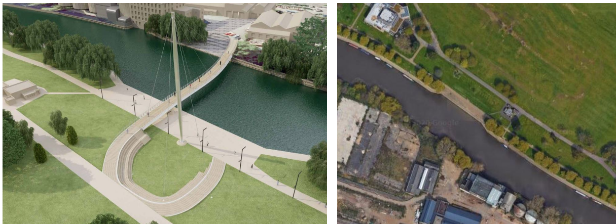
Fig 30 & 31: Pedestrian bridge concept (feasibility stage) and aerial photo showing future proofing to both sides of the riverbank for landing areas
